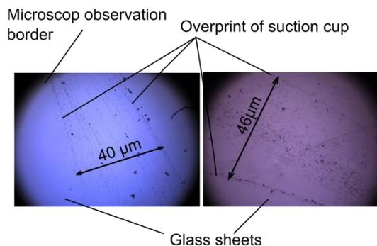
Fig. 3: Overprint on surface of the glass after contact with the suction cup with driving pressure of 3,5 Bar (left) and of 5 Bar (right)
