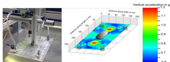
Fig. 12: Maximum vibrations values occurring at the gripper surface
