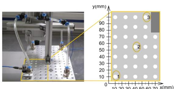
Fig. 5: Observation area of the mounted suction gripper
