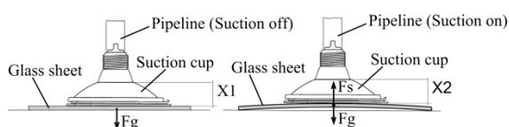
Fig. 2: Value of glass sheet deformation which caused by turning suction on should be kept at the sufficient level.
