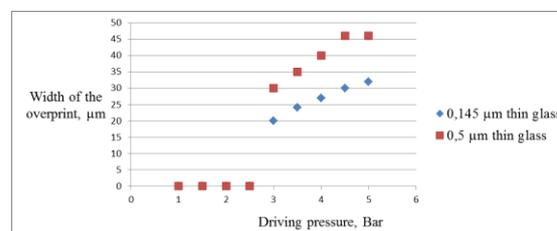
Fig. 4: Overprints width, left by the suction cup during suction process, for range of values of driving pressure
