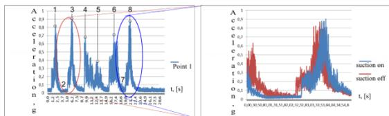
Fig. 9: Image of the maximum vibration values at 1st point and pressure influence on the vibration maximum value
