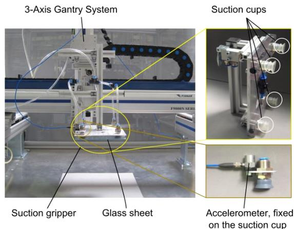
Fig. 1: Constructed Gantry System (left) is equipped with developed suction gripper with suction cups (right above) and accelerometer, fixed directly on the suction cup (right below).
