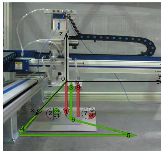
Fig. 7: The movement cycle: the arrows denote the direction of movement at each of the iterations. Green color of arrow signifies the presence of pressure at the system, red – absence.
