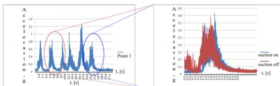
Fig. 11: Image of the maximum vibration values at 3rd point and pressure influence on the vibration maximum value
