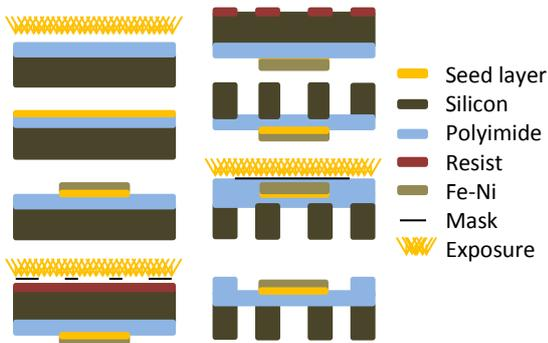
Fig. 8 Processing steps of the first membrane [5]
