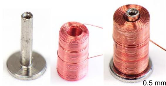
Fig. 6 Softmagnetic Core, Coil and coil attached to the core
