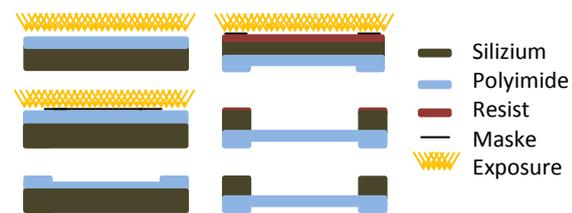
Fig. 9 Processing steps of the second membrane [5]
