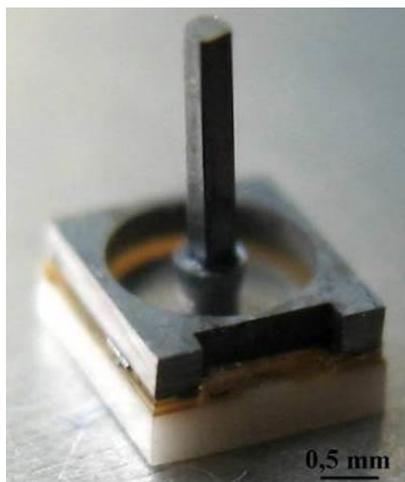
Fig. 4 Completed system of the hearing aid implant [4]
