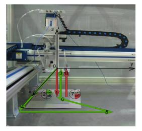
Fig. 7: The movement cycle: the arrows denote the direction of movement at each of the iterations. Green color of arrow signifies the presence of pressure at the system, red – absence.
