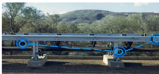
Fig. 2 RFID Node to node communication for conveyor idler monitoring [6]
