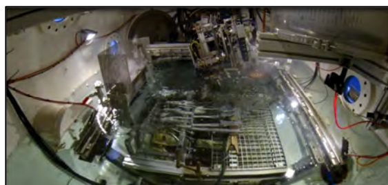
Fig. 18 Bead on plate weld for determination of diffusible hydrogen content
