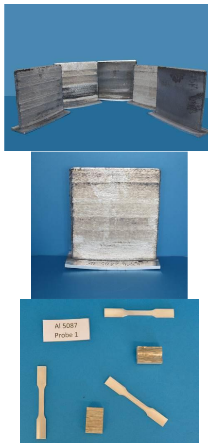
Figure 4: Sample plate circumference per alloy (left); example of a 300x300 mm flat structure made of Al 5087 (middle); representation of the samples taken to perform the mechanical test.
