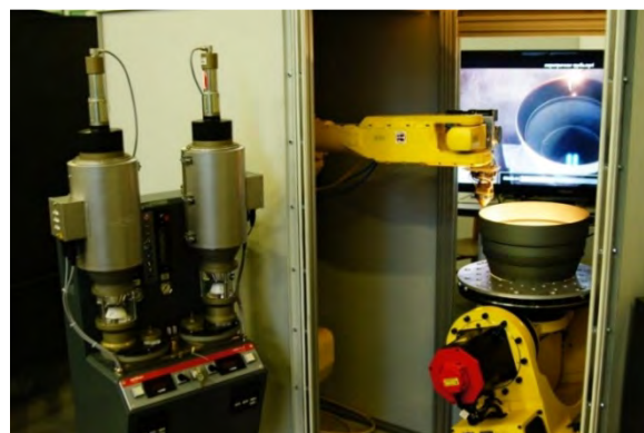
Fig. 1 High-speed direct laser deposition equipment.
