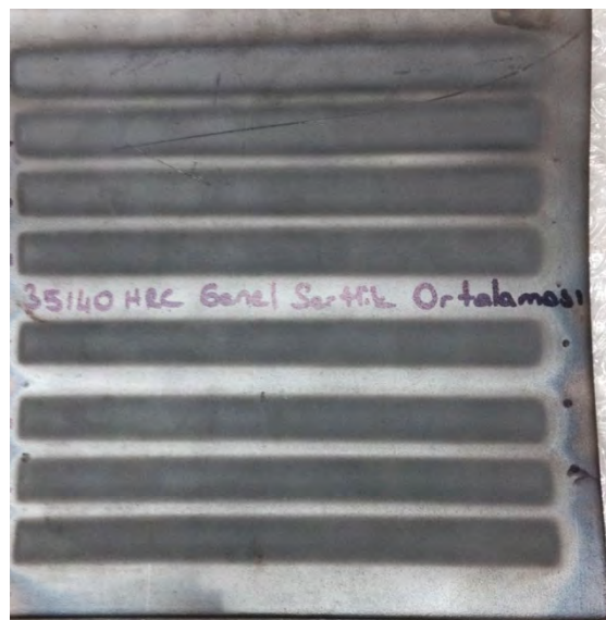
Fig. 4 Laser hardened sheet surface after gas cementation
