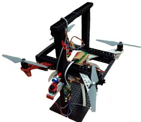
Fig. 3 Sensors identification stand
