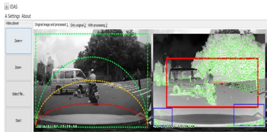
Fig. 4 Results of working software module for predicting danger situations
