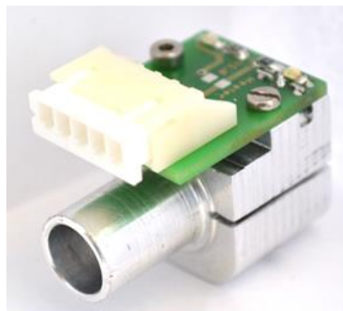
Figure 2 Thermal stabilization module
